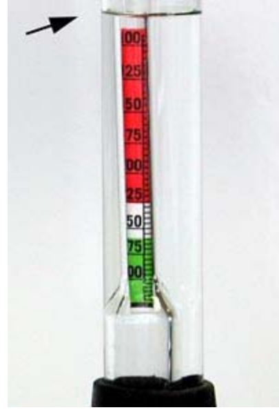
The reading is below 1.100. When compared to the other readings, this indicates a bad cell.
