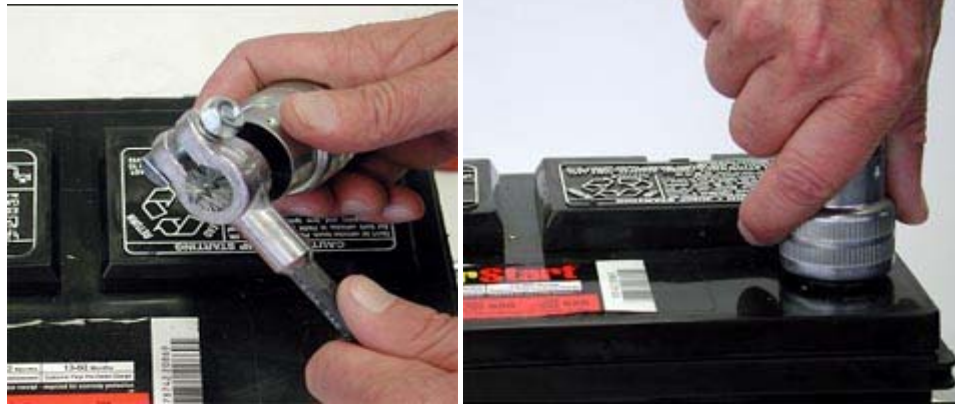
Cleaning Terminals with a Terminal Brush
