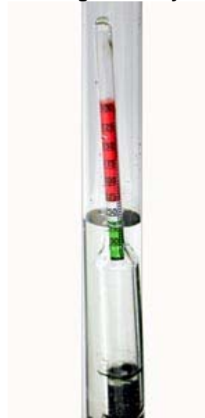
Notice how buoyant the float is in this fully-charged battery
